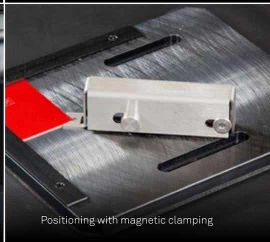
Positioning with magnetic clamping
