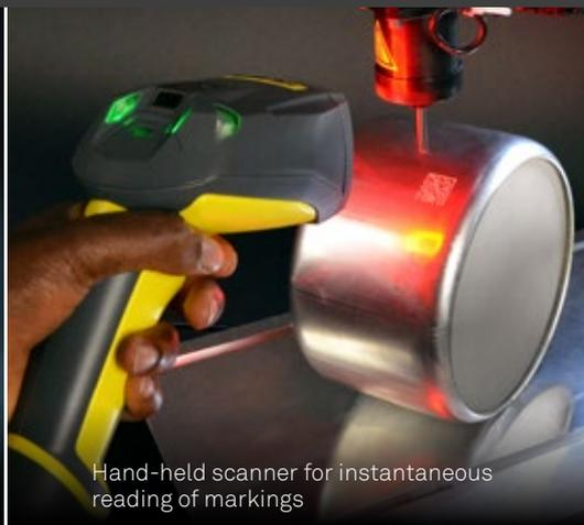
Hand-held scanner for instantaneous reading of markings
